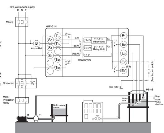
**Note: 1.** Be sure to ground the common Electrode  $E_3$  (the longest Electrode).
