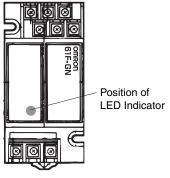
Note: LED indicator is provided on Controllers manufactured in August 1999 or later. It is not mounted on the case surface. It can be seen through the case.
