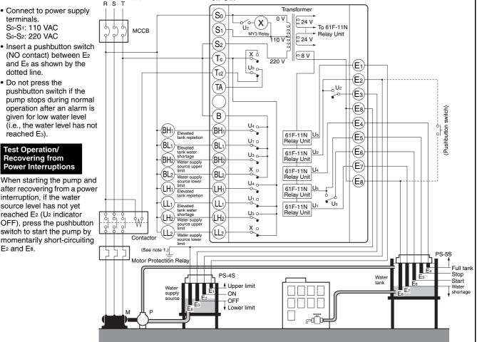
Note: 1. Be sure to ground the common Electrode E8 (the longest Electrode).
