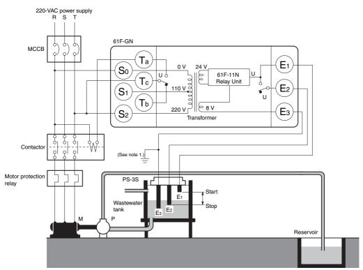
Note: 1. Be sure to ground the common Electrode  $E_3$  (the longest Electrode).
