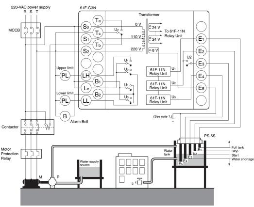
Note: 1. Be sure to ground the common Electrode E<sub>5</sub> (the longest Electrode).
